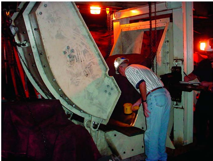
4. Advanced transfer chute hood. According to Benetech, its "Reach" transfer chute is less costly to maintain. Courtesy: Benetech Inc.
